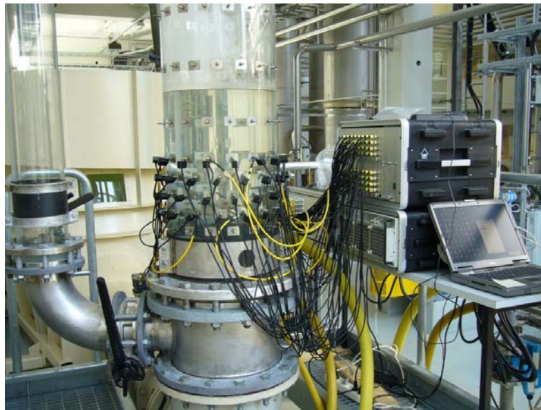
Figure 3: The measurement part of the mixing loop and KIT4 measurement system.
