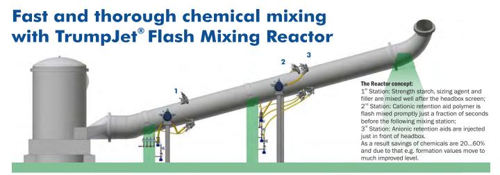
TrumpJet Flash Mixing Reactor mixes numerous additives in a chaos type of pattern efficiently very close to the machine. The system will maximize efficiency of the used additives.
