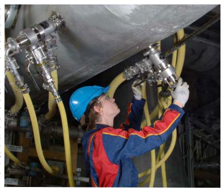
Wetend has developed a new concept where opposite charge chemicals or pairs of chemicals can be mixed in a single reactor zone with good results. The technology provides an opportunity to i.e. maintain generated filler-fiber composite and flock structures intact before forming and dewatering. It also enables the use of aggressive additives as well as develop composite structures for the web. This is
