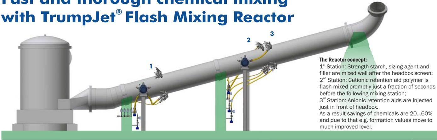
TrumpJet Flash Mixing Reactor mixes numerous additives in a chaos type of pattern efficiently very close to the machine. The system will maximize efficiency of the used additives.
