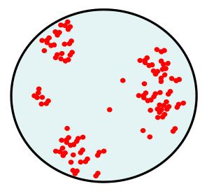
Bad/Poor dispersion, Bad/Poor distribution
